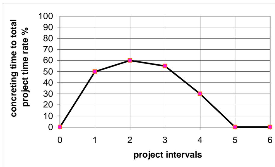
**Figure-1.** Concreting process duration relative to total project duration rate.
