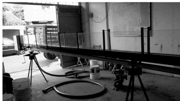
Photo 2. Hydraulic jack, tripods and energy dissipation tank (Prepared by the author, 2018)
